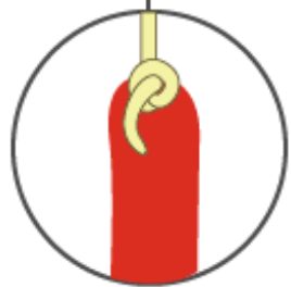
The string with a tag for attracting the animal into pulling it, to lift the bolt from the ring.
