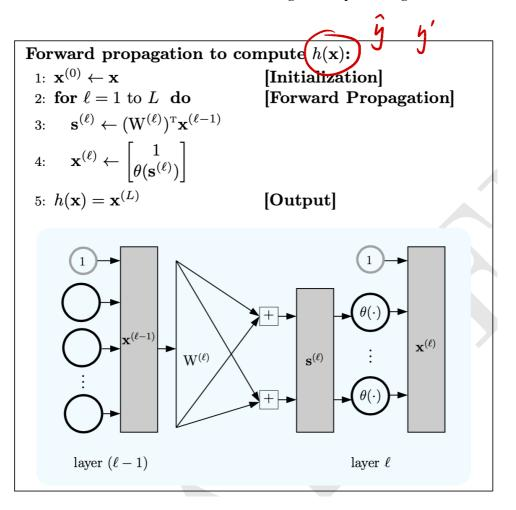
After forward propagation, the output vector  $\mathbf{x}^{(l)}$  at every layer l = 0, 1, 2, ..., L has been computed.
