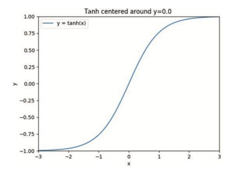
The hyperbolic tangent function maps x from  $(-\infty, +\infty)$  to y in the range of [-1, 1]. It is a soft version of bipolar step function we used for perceptron.
