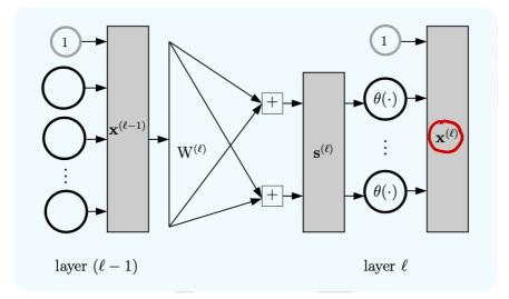
The neural network hypothesis  $h(\mathbf{x})$  is computed by the forward propagation algorithm. First observe that the inputs and outputs of a layer are related by the activation function,
