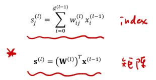
All that remains is to initialize the input layer to  $\mathbf{x}^{(0)} = \mathbf{x}$  (so  $d^{(0)} = d$ , the input dimension) and use the above equations in the following chain,
