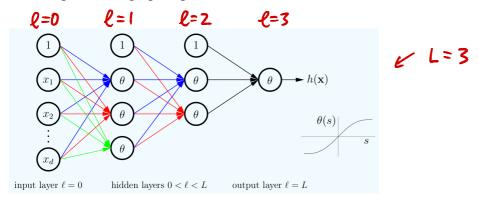
While this graphical view is aesthetic and intuitive, with information *flowing* from the inputs on the far left, along links and through hidden nodes, ultimately to the output  $h(\mathbf{x})$  on the far right, it will be necessary to algorithmically describe the function being computed. Things are going to get messy, and this calls for a very systematic notation; bear with me.
