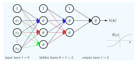
For the most part, we only need to deal with the network on a layer by layer basis, so we introduce vector and matrix notation for that. We collect all the input signals to nodes  $1, 2, ..., d^{(l)}$  in layer l in the vector  $\mathbf{s}^{(l)}$ . Similarly, collect the output from nodes  $0, 1, 2, ..., d^{(l)}$  in the vector  $\mathbf{x}^{(l)}$ .
