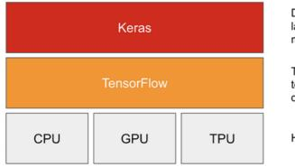
Deep learning development: layers, models, optimizers, losses, metrics... Tensor manipulation infrastructure: tensors, variables, automatic differentiation, distribution... Hardware: execution
