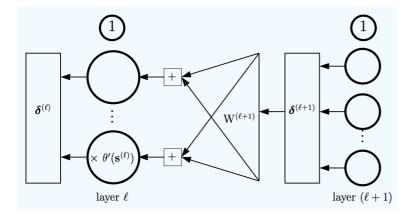
In the figure, layer (l + 1) outputs (backwards) the sensitivity vector  $\delta^{(l+1)}$ , which gets multiplied by the weights  $\mathbf{W}^{(l+1)}$ , summed and passed into the node in layer l multiply by  $\theta'(\mathbf{s}^{(l)})$  to get  $\delta^{(l)}$ . Using component-wise multiplication  $\otimes$ , a shorthand notation for this backpropagation step is:
