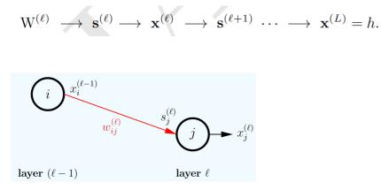
To derive (1), we drill down to a single weight and use the chain rule. For a single weight  $w_{ij}^{(l)}$ , a change in  $w_{ij}^{(l)}$  only affect  $s_j^{(l)}$  and so by the chain rule:
