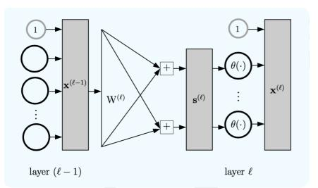
The outputs  $\mathbf{x}^{(l)}$  for every layer  $l \ge 0$  can be computed by a forward propagation. So to get the partial derivatives, it suffices to obtain the sensitivity vectors  $\mathbf{\delta}^{(l)}$  for every layer  $l \ge 1$  (remember that there is no input signal  $\mathbf{s}^{(0)}$ ).
