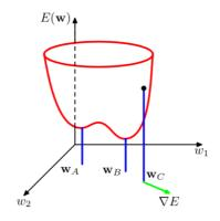
The gradient descent method is a first-order iterative optimization algorithm for finding the minimum of a function. To find a local minimum of a function using gradient descent, one takes steps proportional to the negative of the gradient. We initialize the weights to w(0) and for t = 1, 2, ... update the weights by taking a step in the negative gradient direction,
